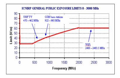
For example, for a GSM mobile signal on a frequency of 940.050 MHz, the relevant limit is 42.158 V/m, while for a 3G mobile signal on a frequency of 2147.2 MHz the relevant limit is 61 V/m. Thus the limits for the different measurements presented in the tables will vary as the measurements have been performed at different frequencies.
