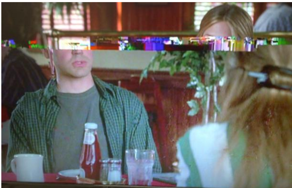
Figure C-5 – Disruption to DTT signal as a result of RF overload in the presence of LTE signal.
