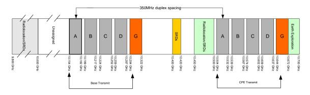
Figure 1: FWALA channel arrangements in the 10.5 GHz band (nationwide, excluding Dublin and Cork)
