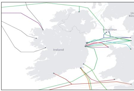
Figure 5: Submarine cables connecting to the Island of Ireland
