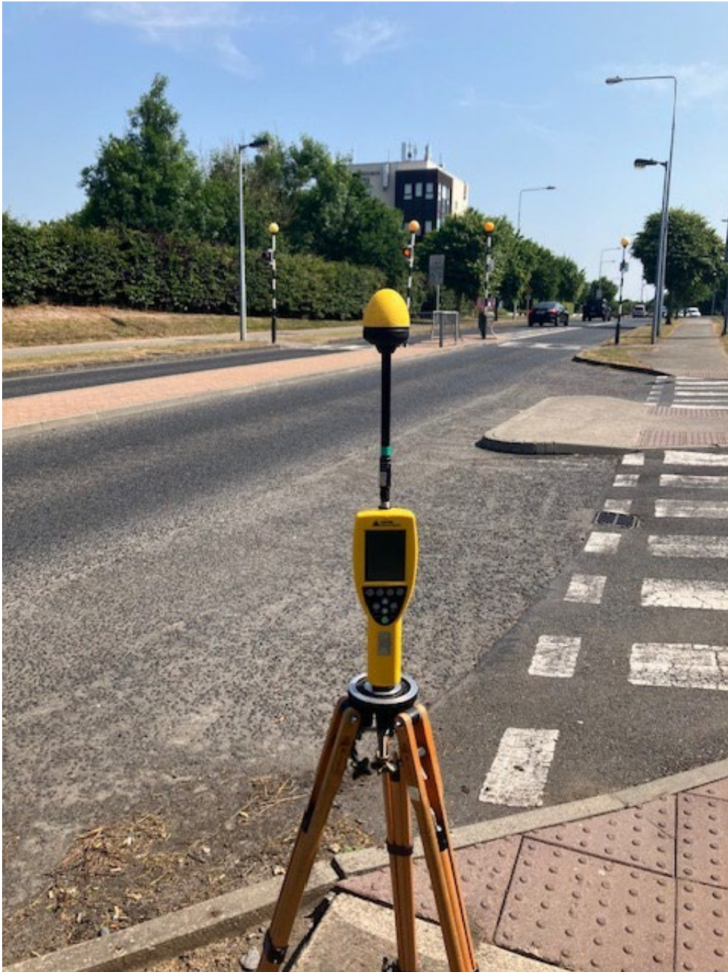
Photo 1. Broadband Measurement location looking towards antennas
