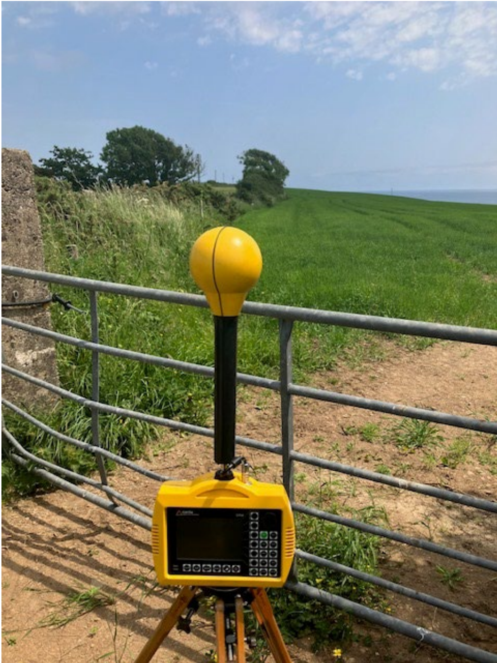
Photo 2. Frequency selective measurement location looking towards antennas
