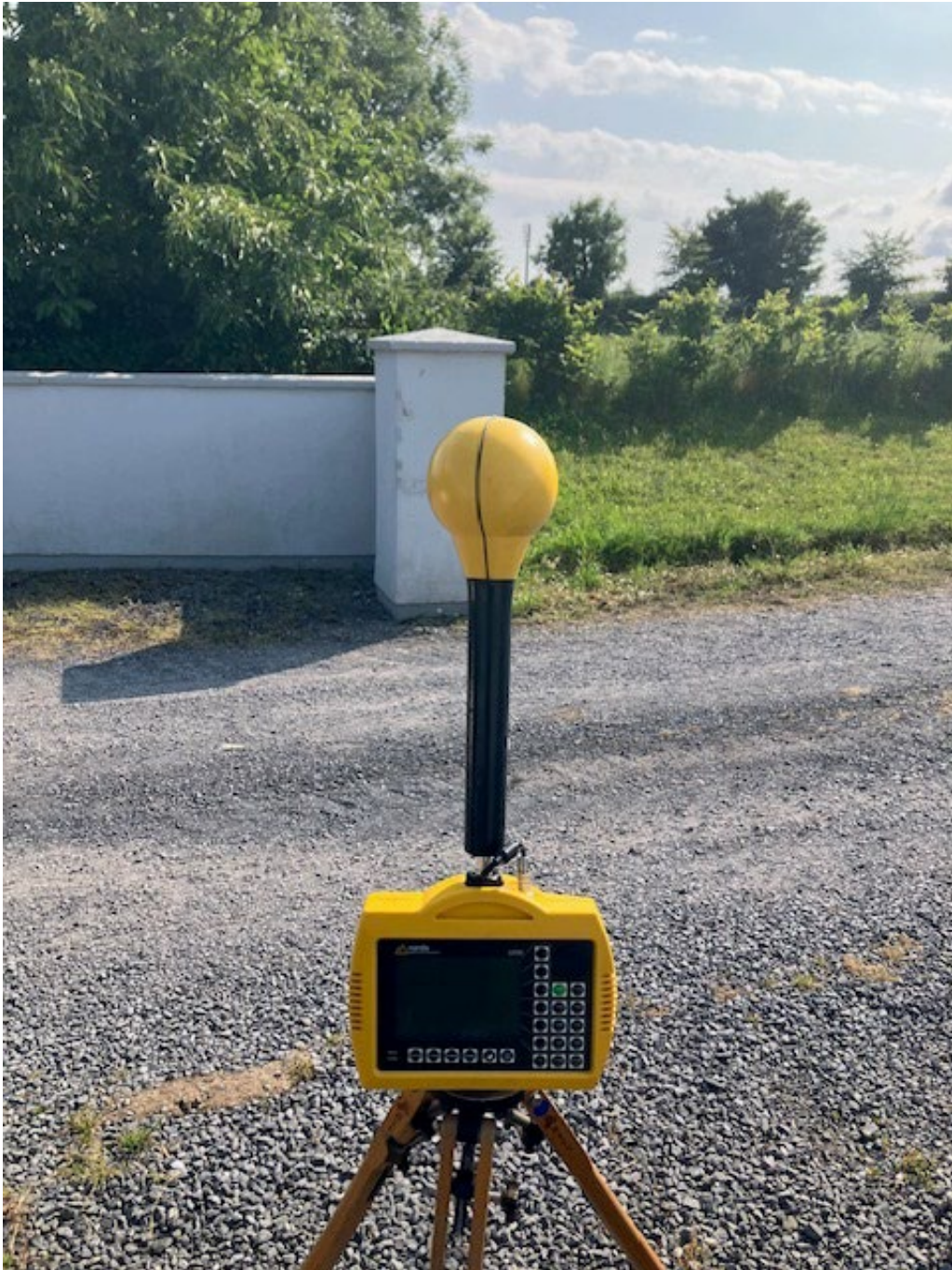
Photo 2. Frequency selective measurement location looking towards antennas
