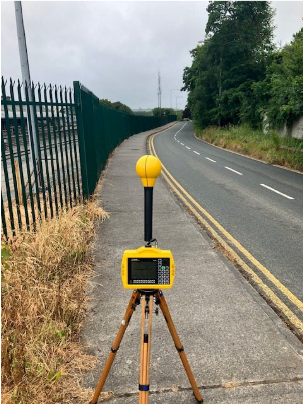
Photo 2. Frequency selective measurement location looking towards antennas
