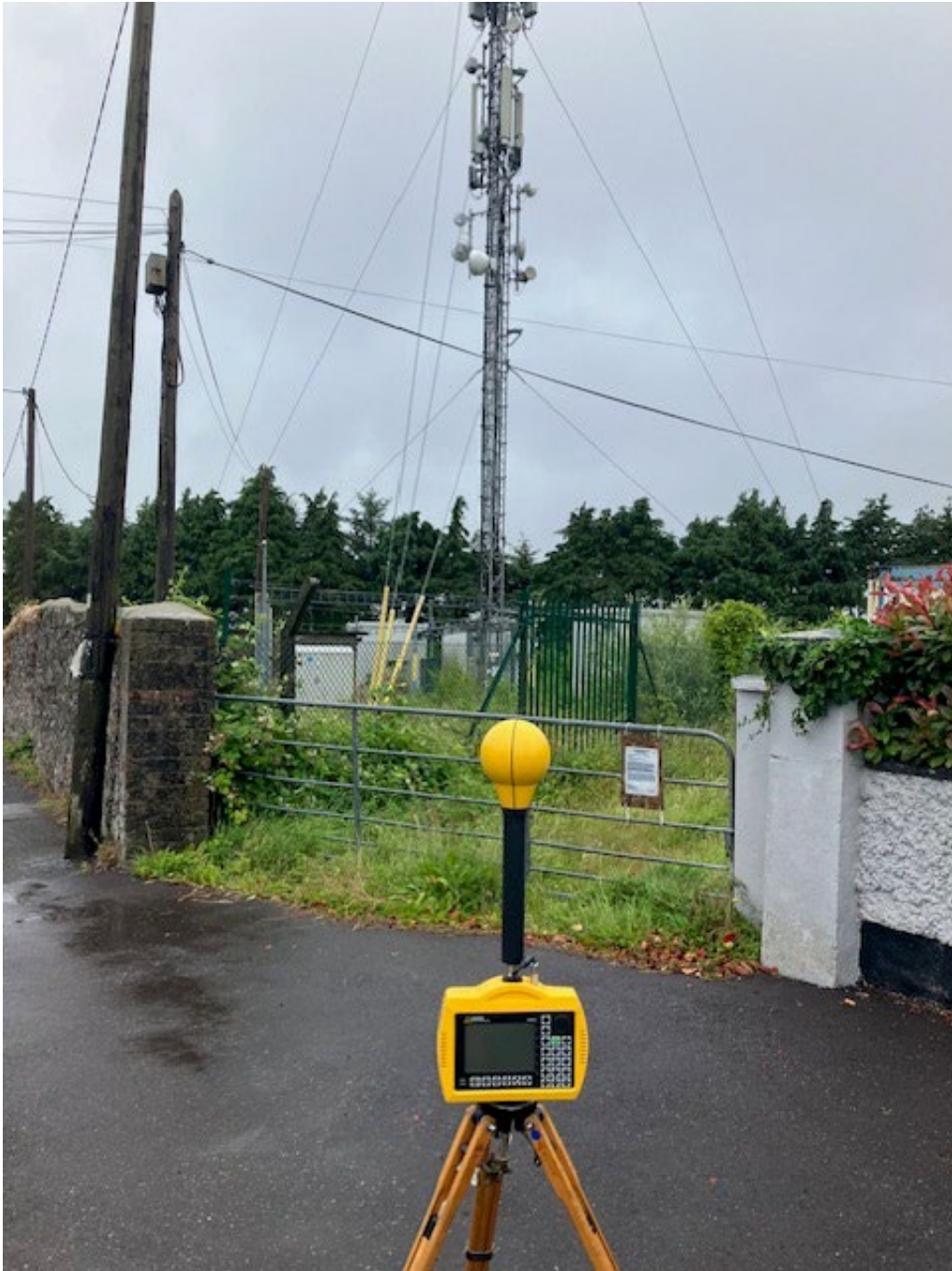
Photo 2. Frequency selective measurement location looking towards antennas
