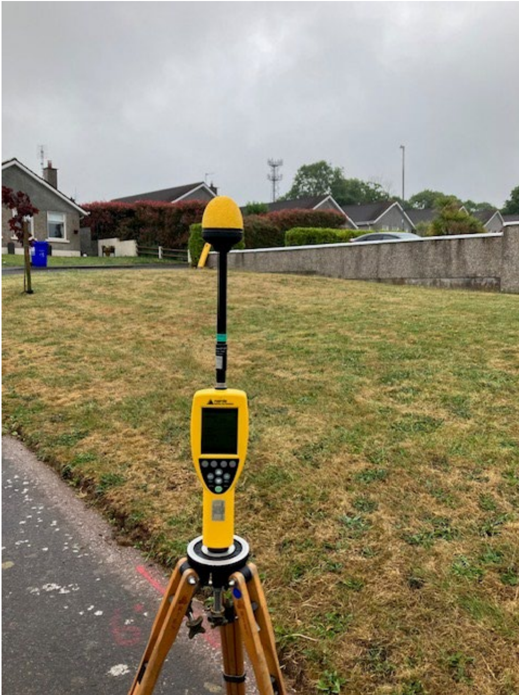
Photo 1. Broadband Measurement location looking towards antennas
