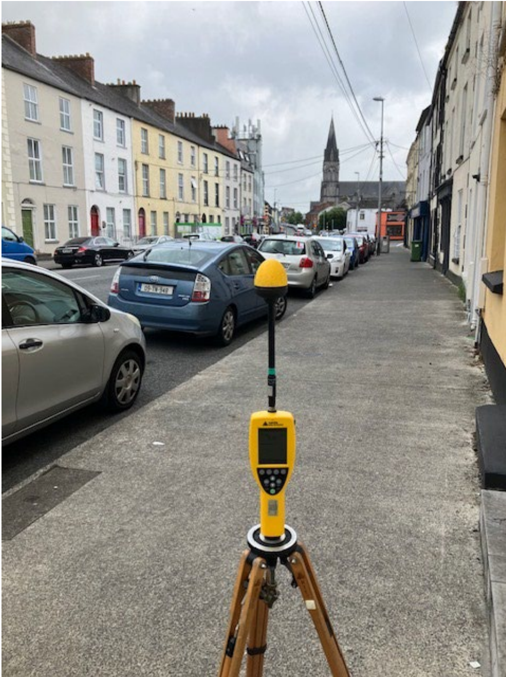
Photo 1. Broadband Measurement location looking towards antennas
