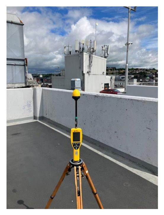
Photo 1. Broadband Measurement location looking towards antennas
