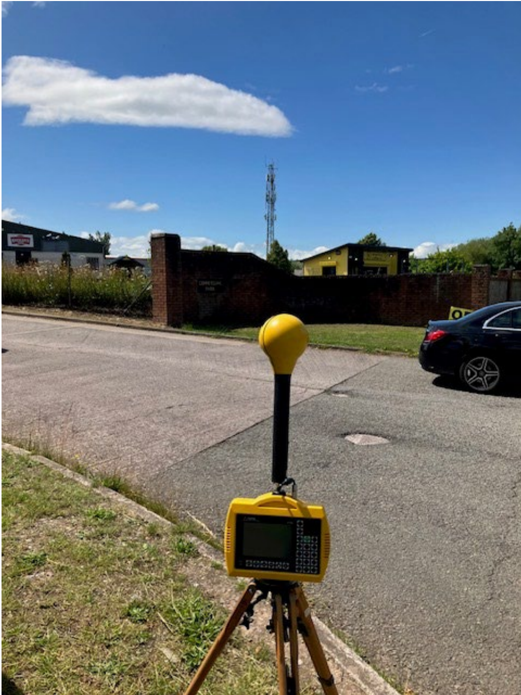
Photo 2. Frequency selective measurement location looking towards antennas
