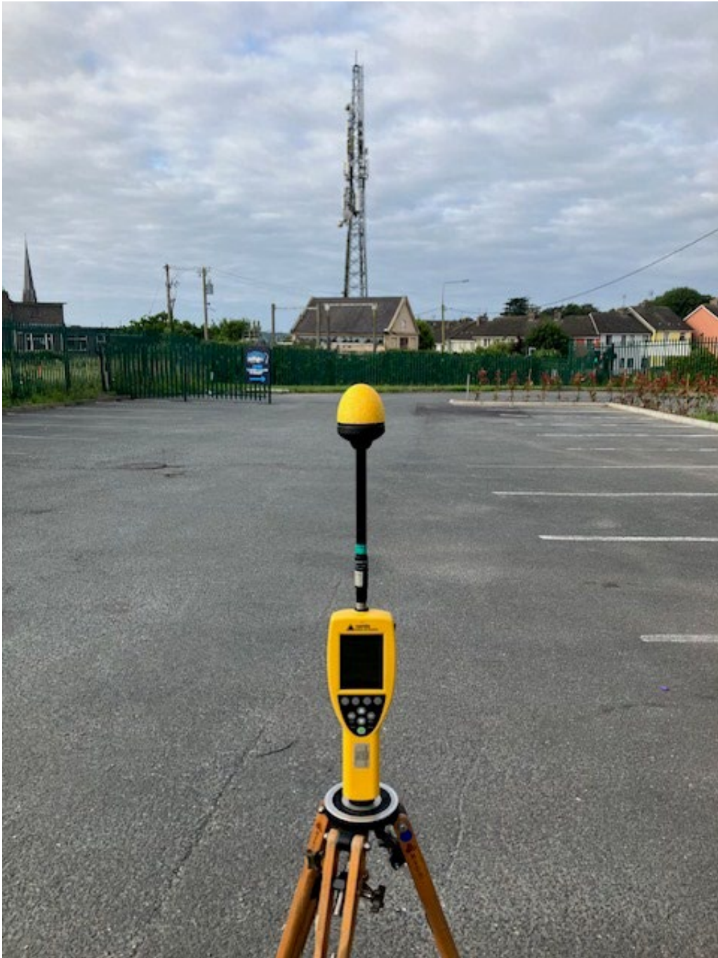
Photo 1. Broadband Measurement location looking towards antennas
