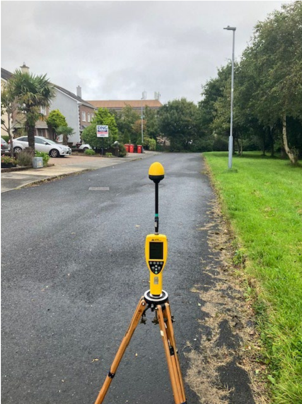
Photo 1. Broadband Measurement location looking towards antennas
