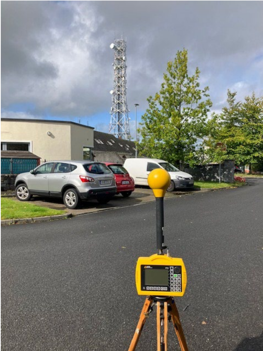
Photo 2. Frequency selective measurement location looking towards antennas
