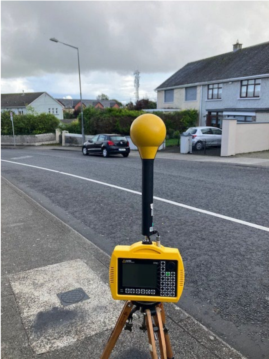
Photo 2. Frequency selective measurement location looking towards antennas
