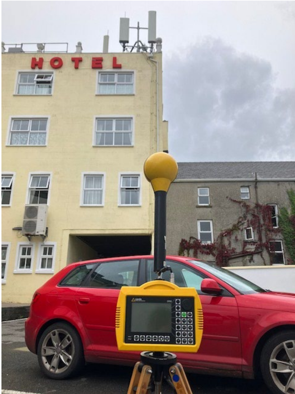
Photo 2. Frequency selective measurement location looking towards antennas
