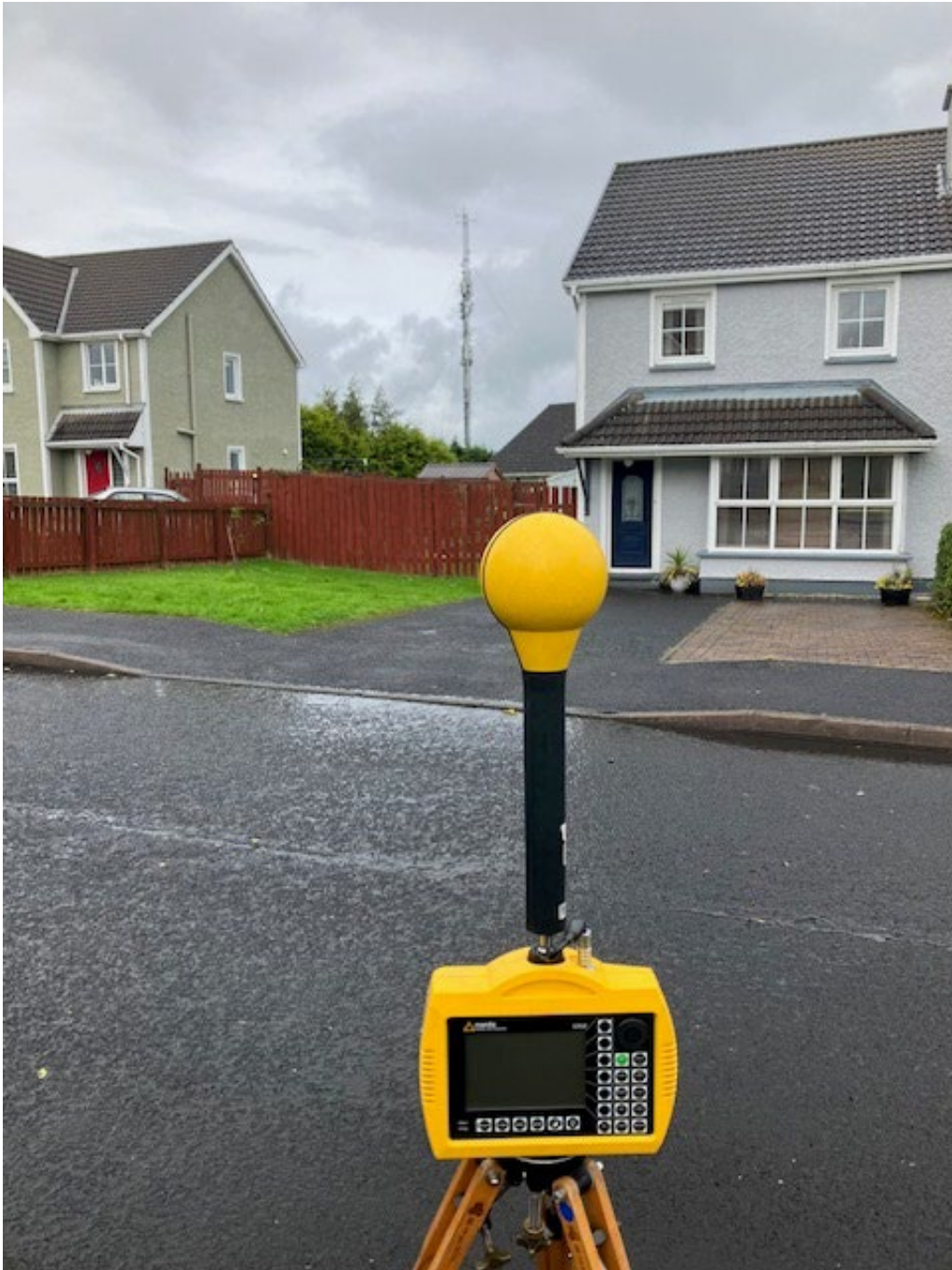
Photo 2. Frequency selective measurement location looking towards antennas
