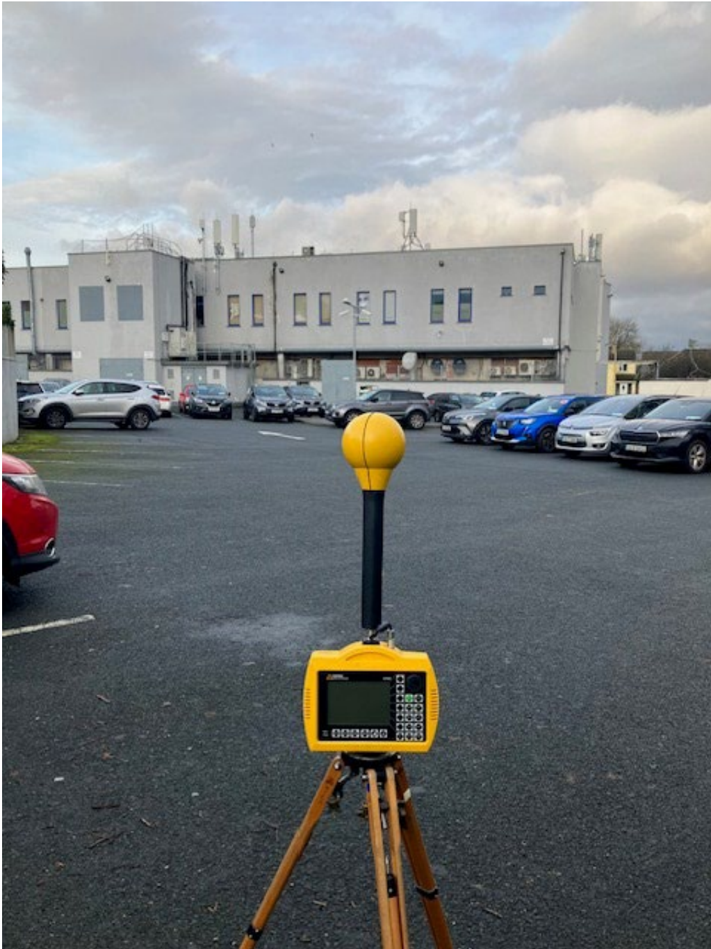
Photo 2. Frequency selective measurement location looking towards antennas
