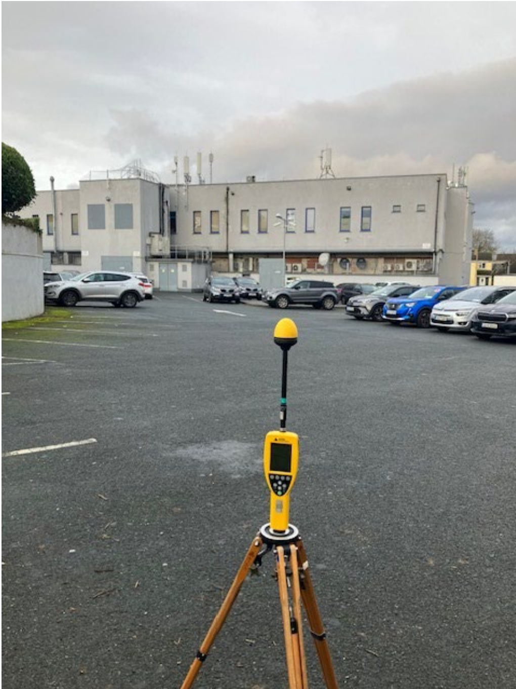
Photo 1. Broadband Measurement location looking towards antennas
