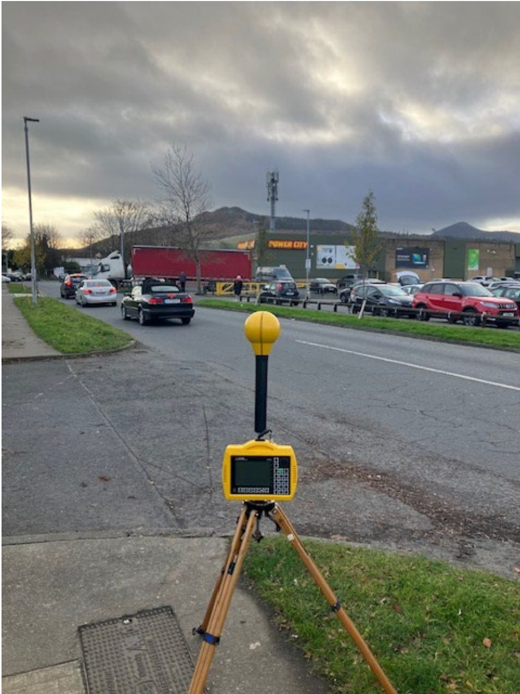
Photo 2. Frequency selective measurement location looking towards antennas
