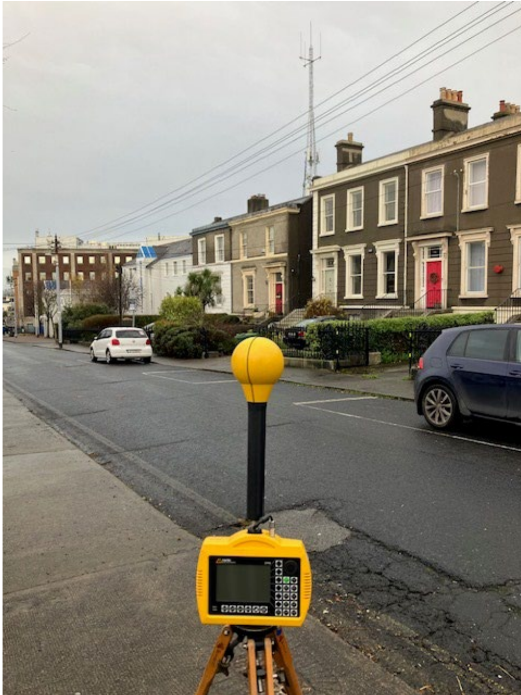
Photo 2. Frequency selective measurement location looking towards antennas
