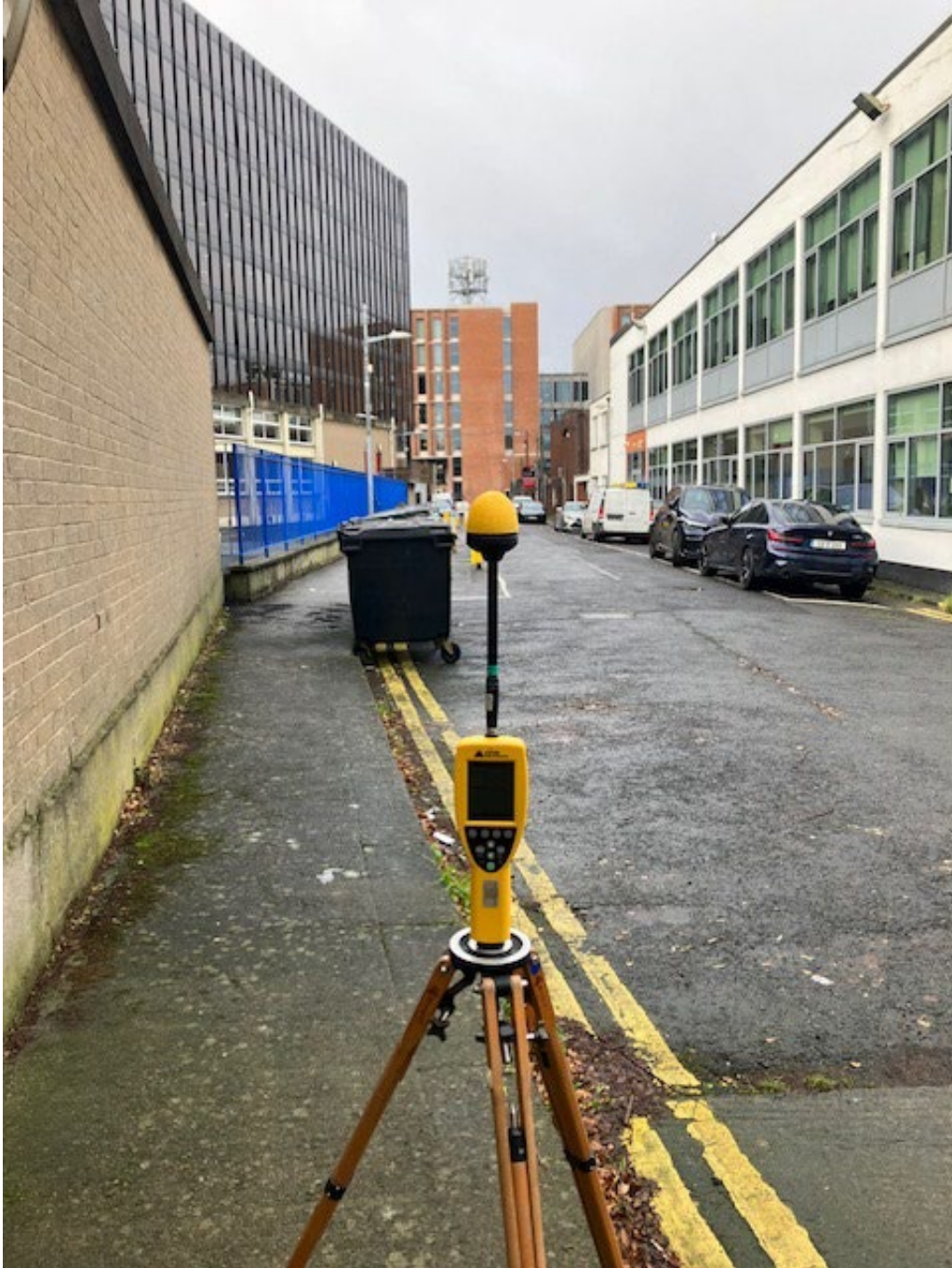
Photo 1. Broadband Measurement location looking towards antennas
