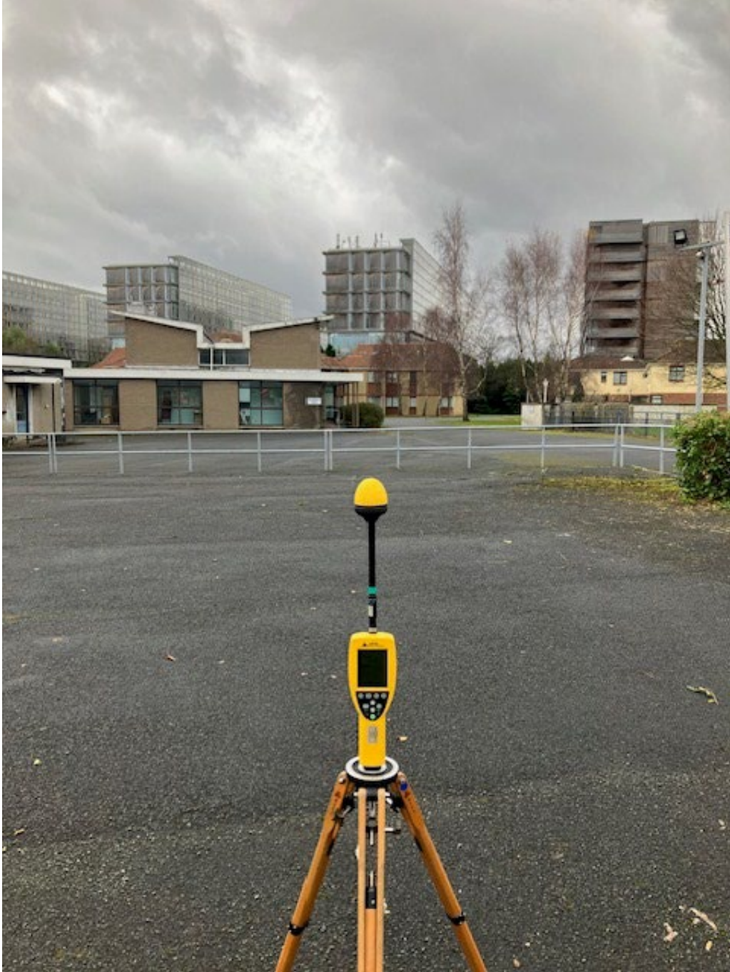
Photo 1. Broadband Measurement location looking towards antennas
