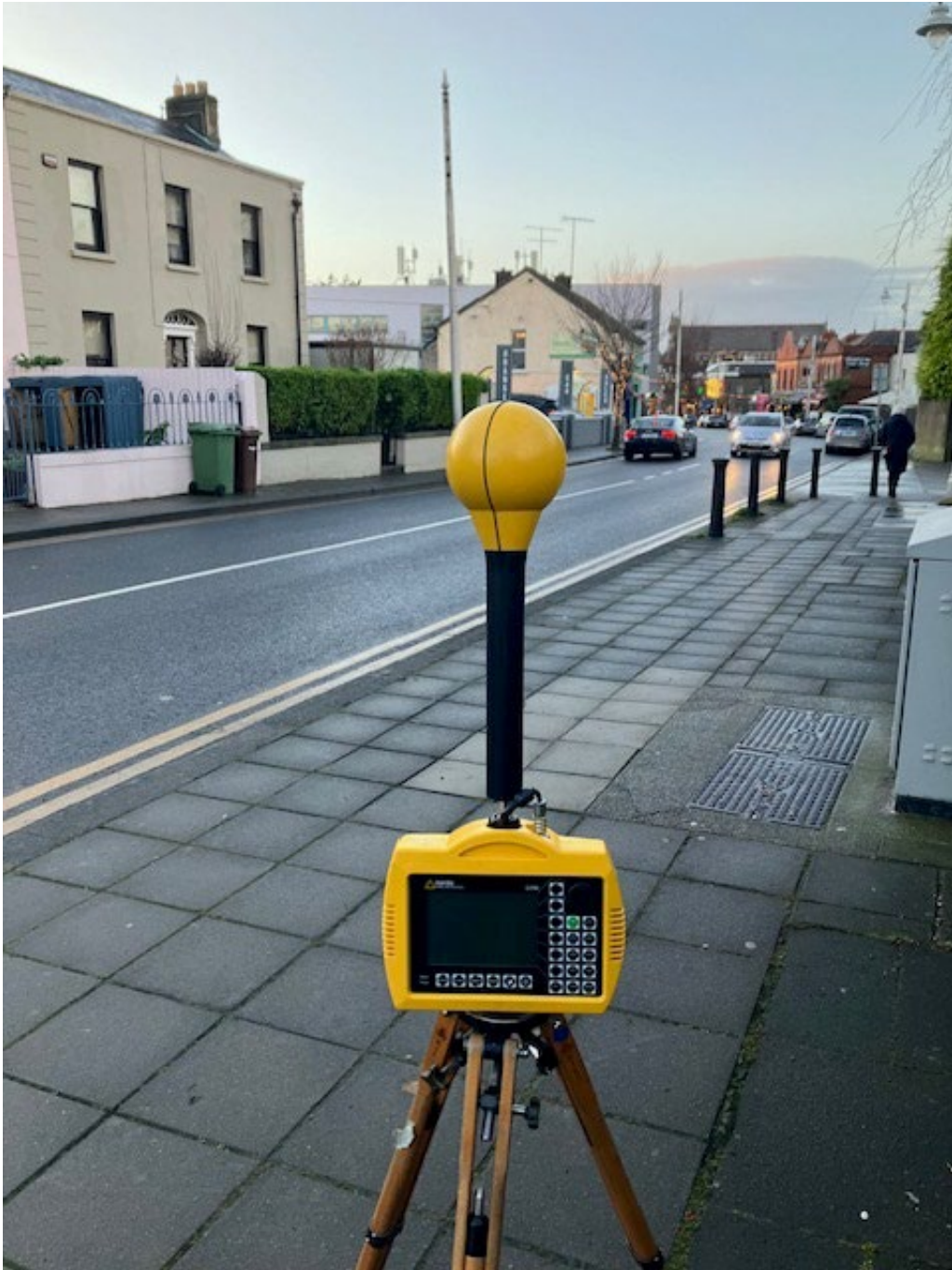
Photo 2. Frequency selective measurement location looking towards antennas
