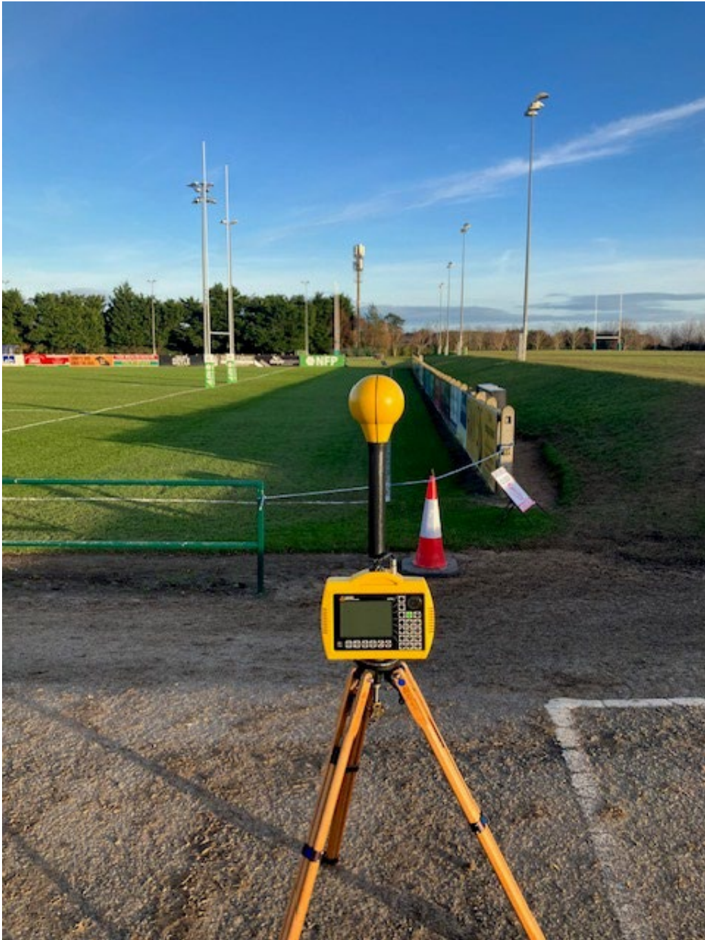
Photo 2. Frequency selective measurement location looking towards antennas
