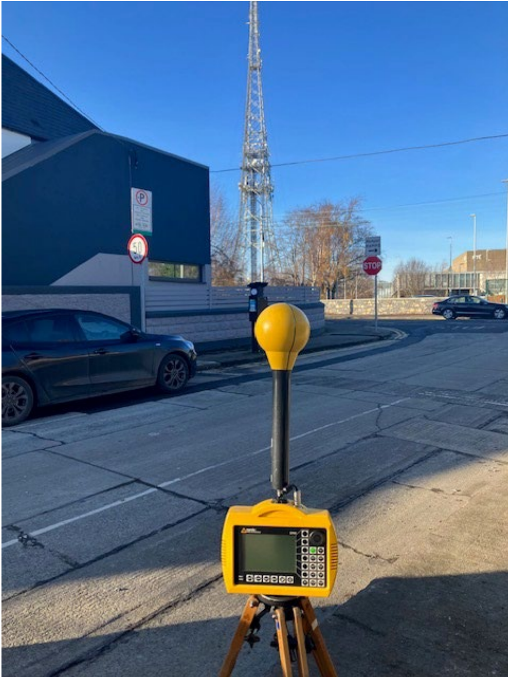
Photo 2. Frequency selective measurement location looking towards antennas
