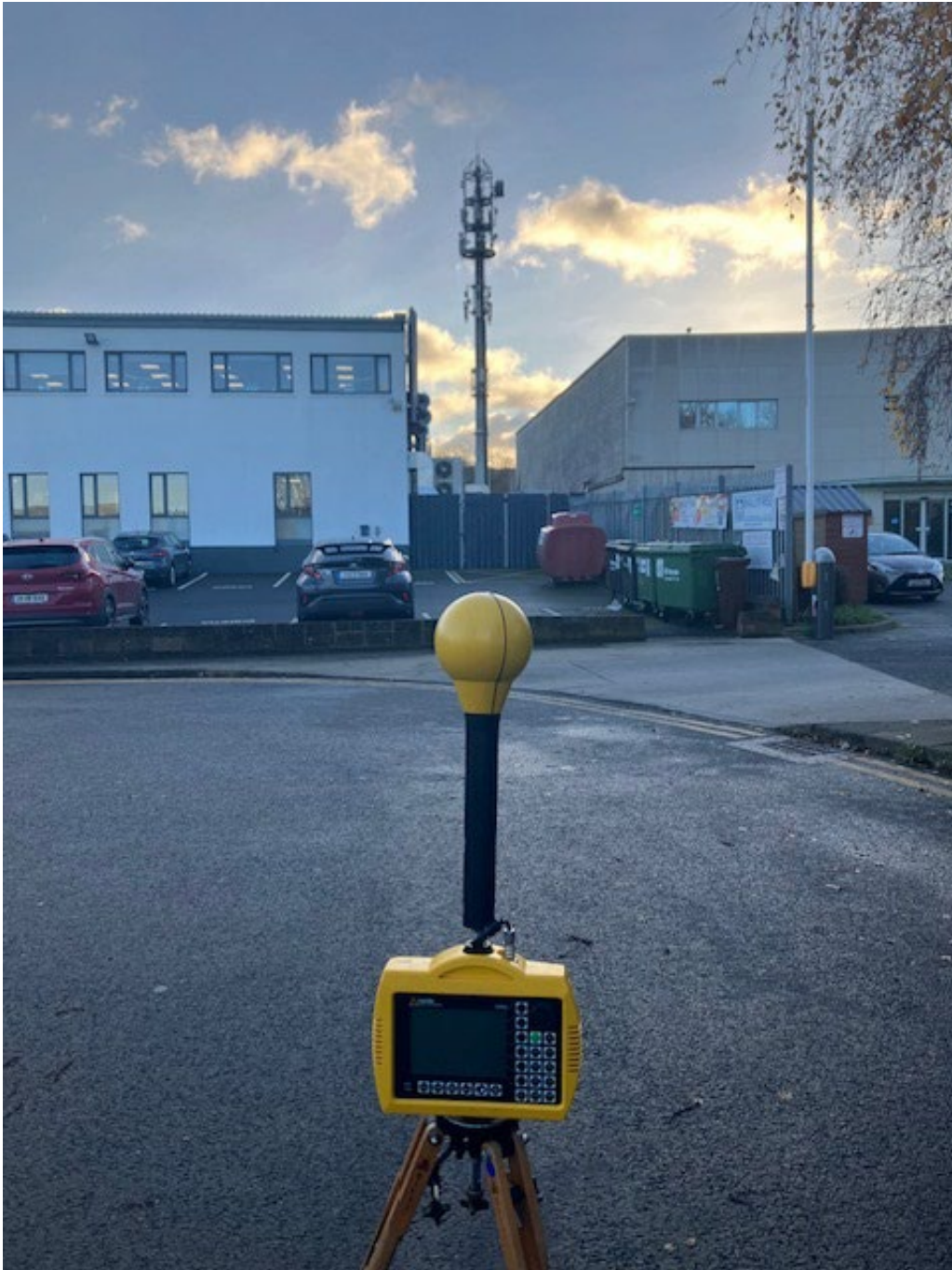
Photo 2. Frequency selective measurement location looking towards antennas
