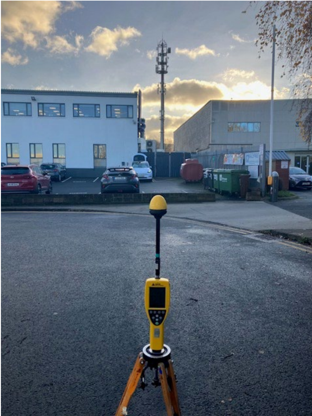
Photo 1. Broadband Measurement location looking towards antennas
