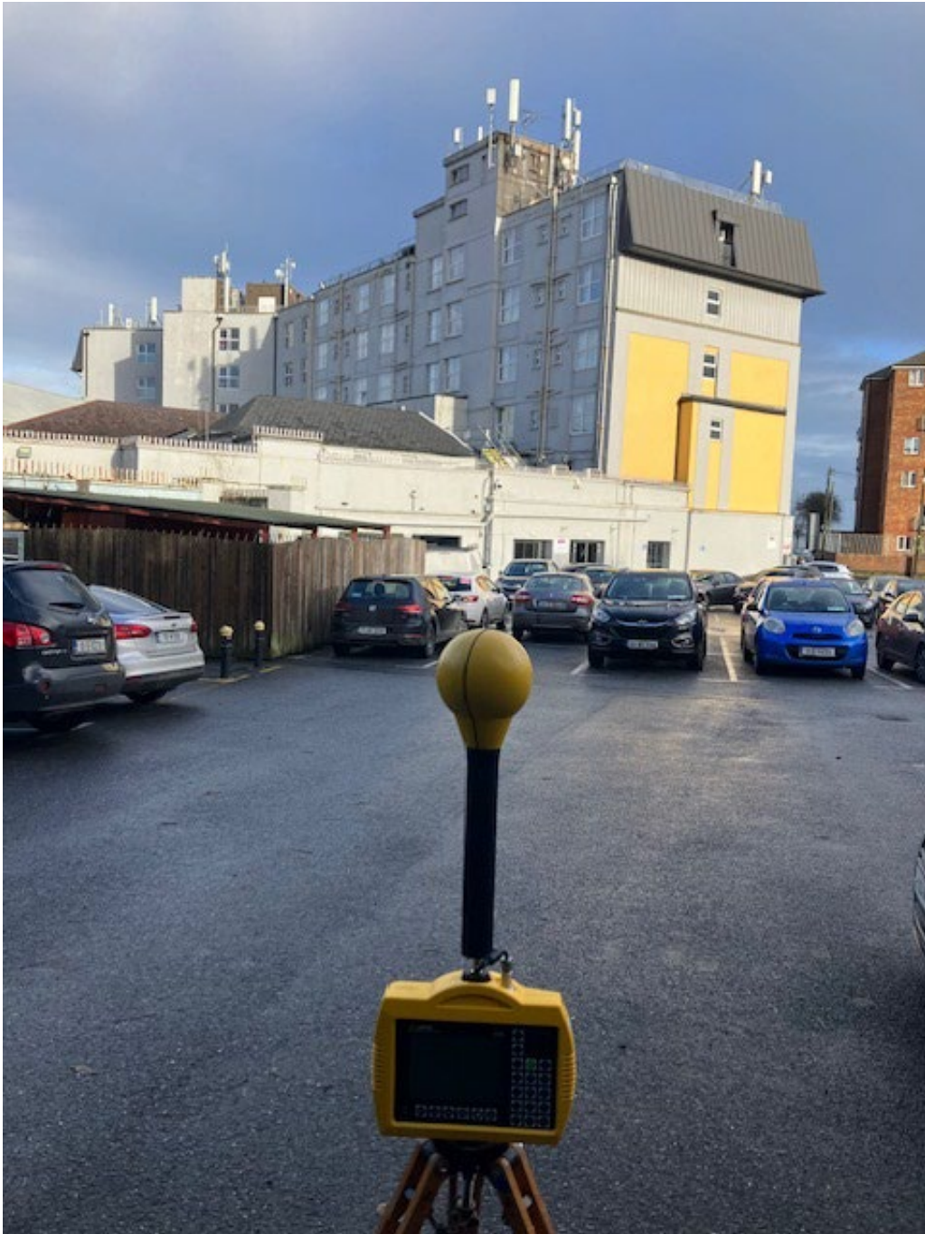
Photo 2. Frequency selective measurement location looking towards antennas
