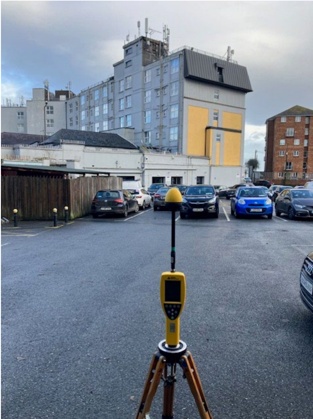
Photo 1. Broadband Measurement location looking towards antennas
