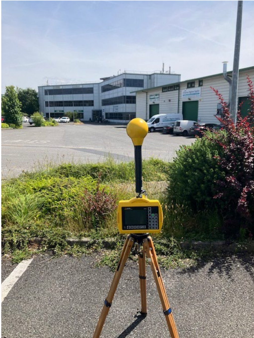
Photo 2. Frequency selective measurement location looking towards antennas
