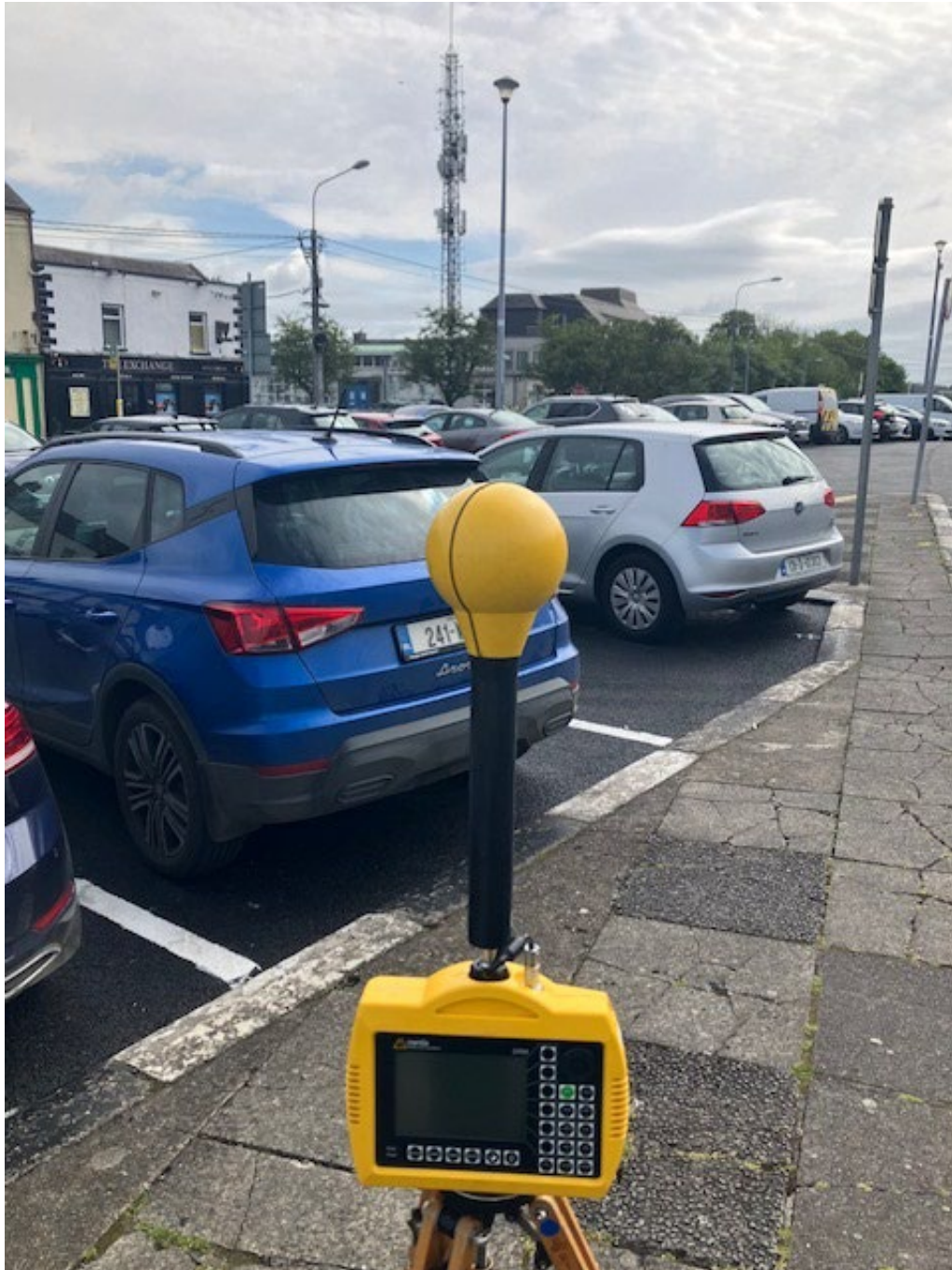
Photo 2. Frequency selective measurement location looking towards antennas
