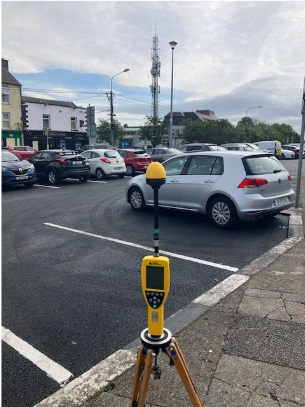
Photo 1. Broadband Measurement location looking towards antennas
