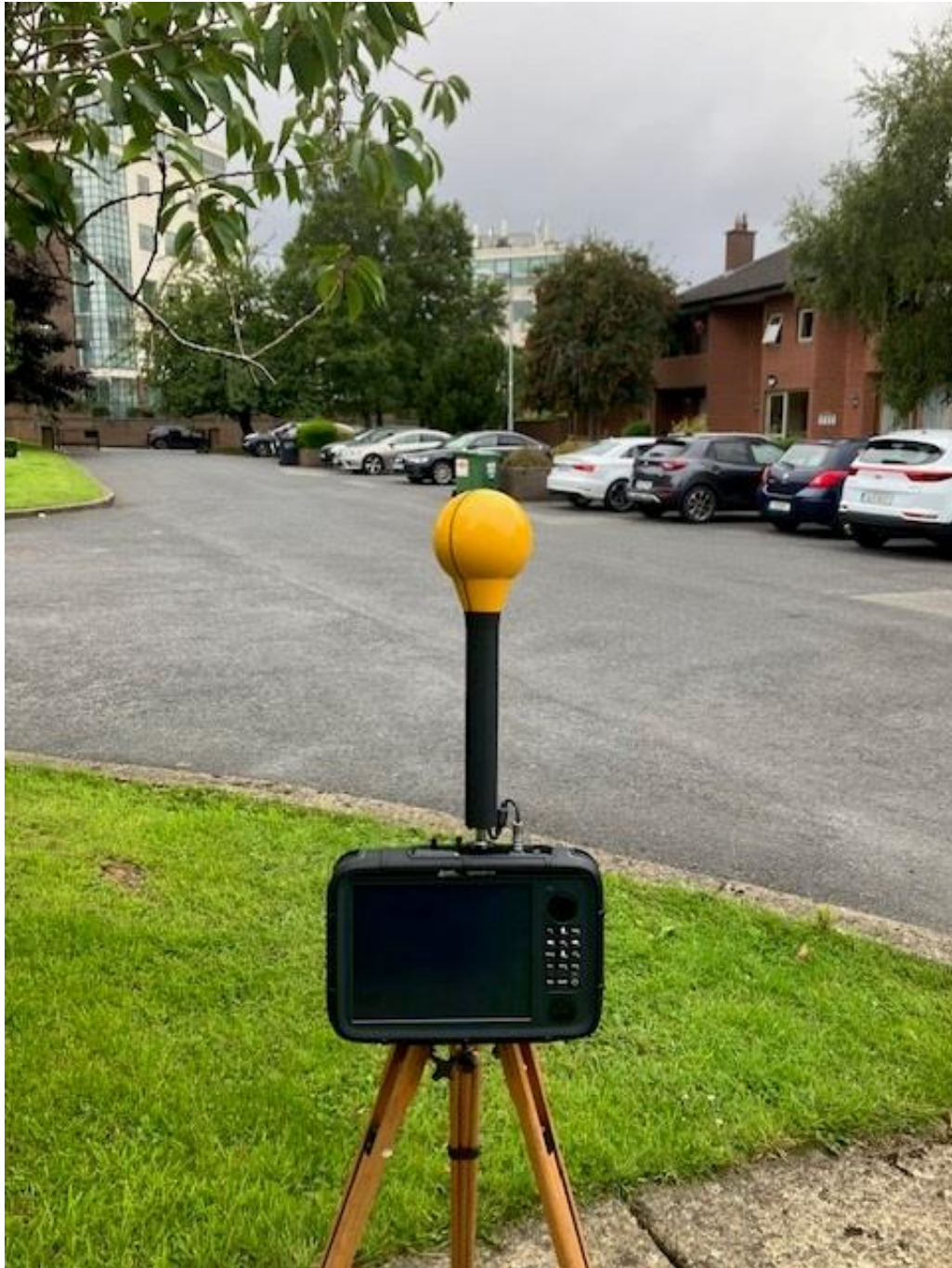
Photo 2. Frequency selective measurement location looking towards antennas
