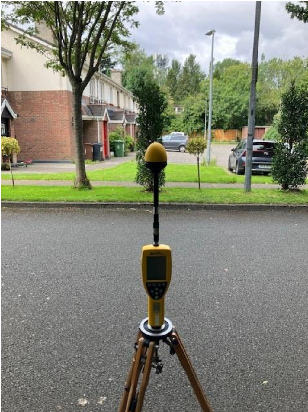
Photo 1. Broadband Measurement location looking towards antennas
