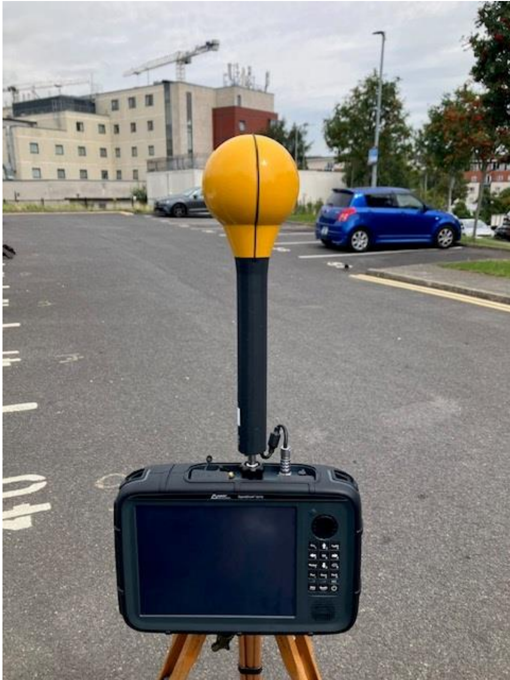
Photo 2. Frequency selective measurement location looking towards antennas
