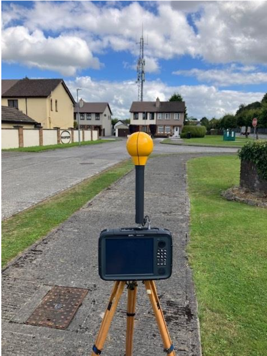
Photo 2. Frequency selective measurement location looking towards antennas
