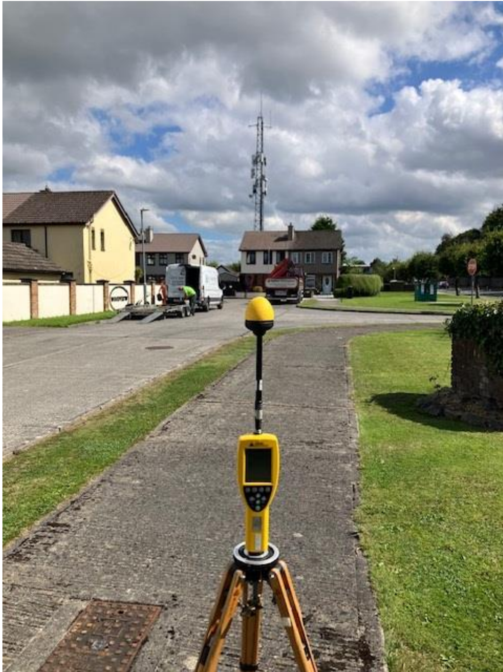
Photo 1. Broadband Measurement location looking towards antennas
