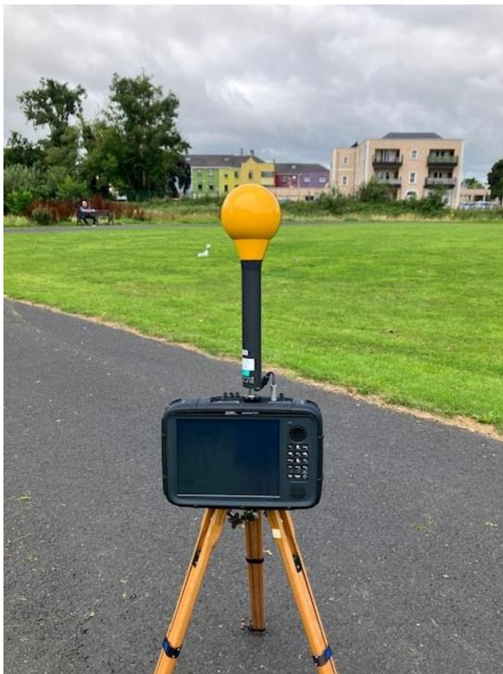
Photo 2. Frequency selective measurement location looking towards antennas
