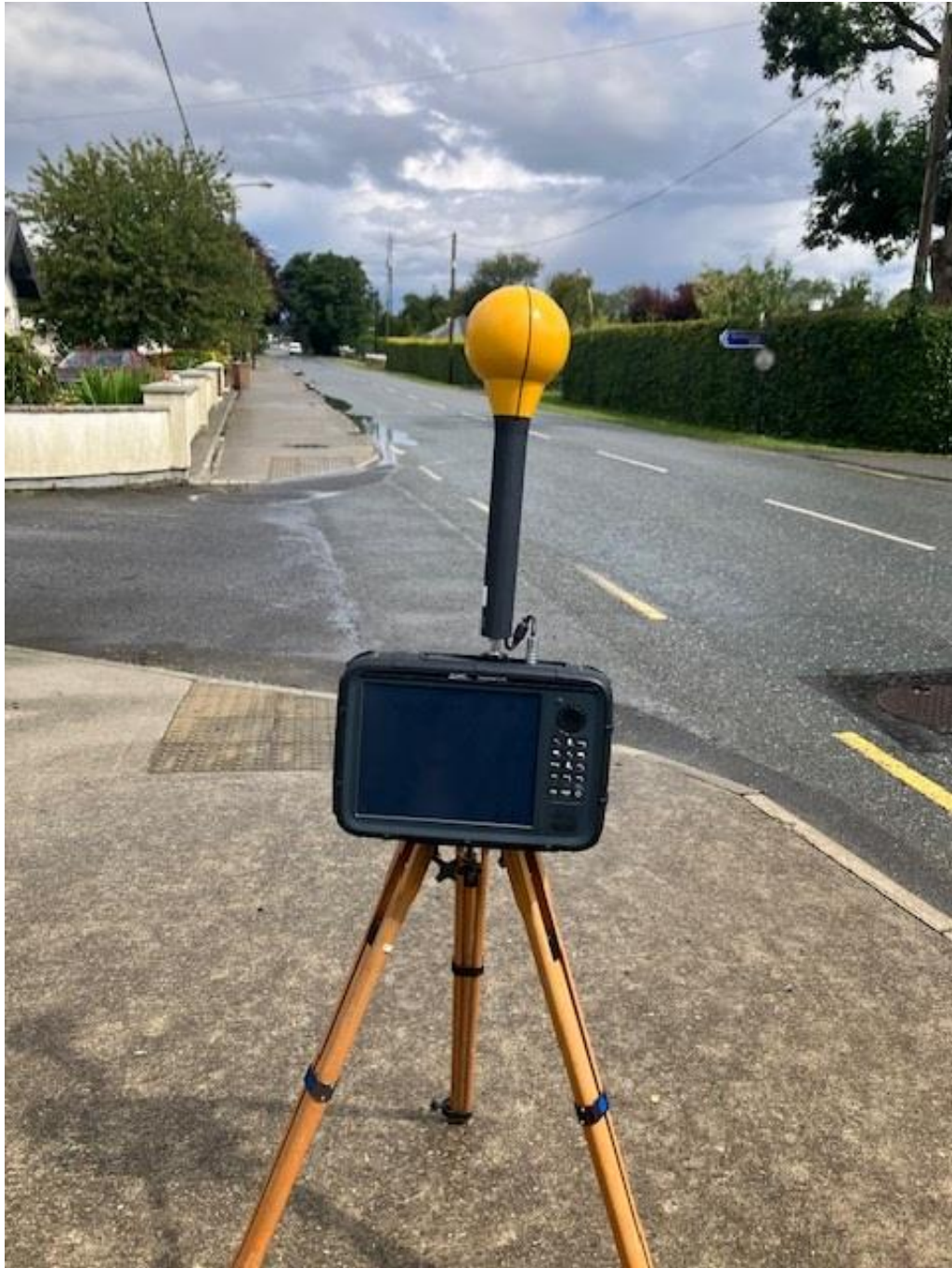
Photo 2. Frequency selective measurement location looking towards antennas
