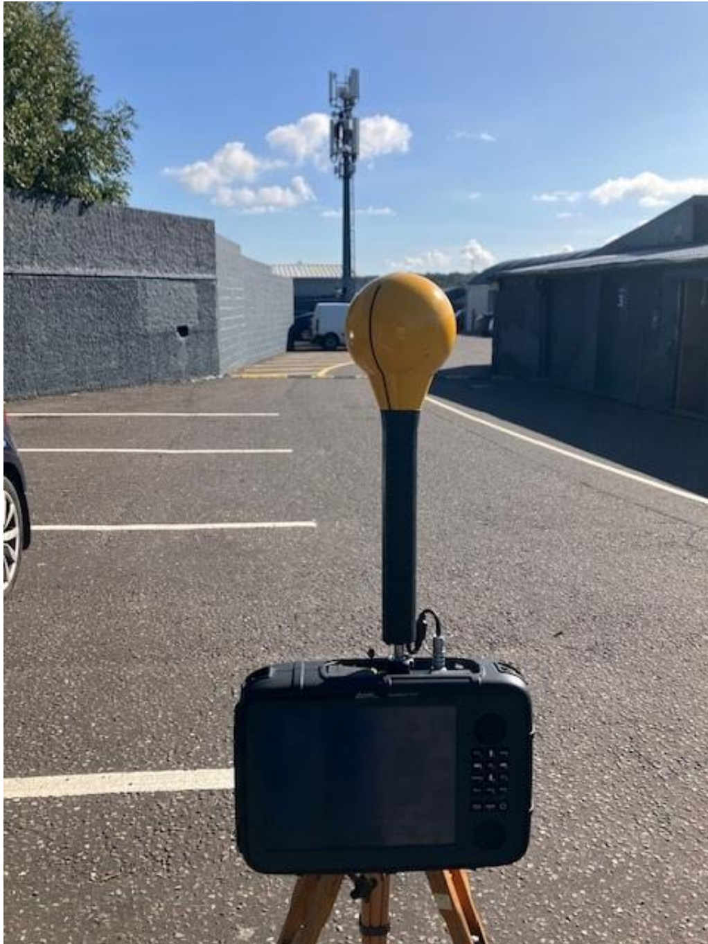
Photo 2. Frequency selective measurement location looking towards antennas
