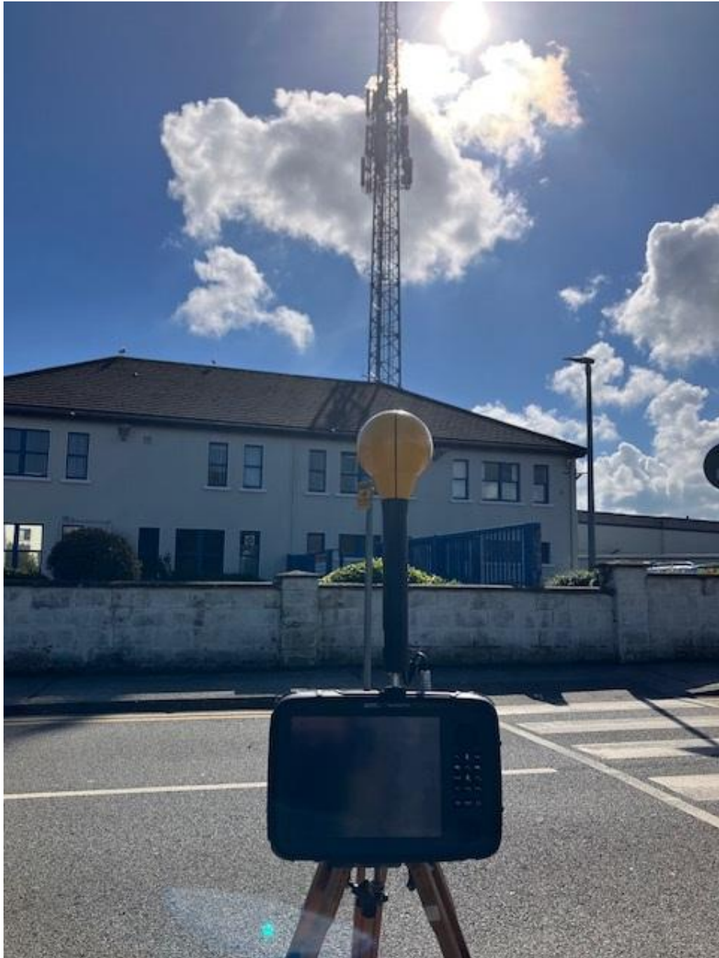
Photo 2. Frequency selective measurement location looking towards antennas
