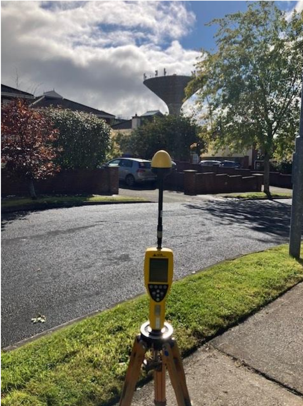
Photo 1. Broadband Measurement location looking towards antennas
