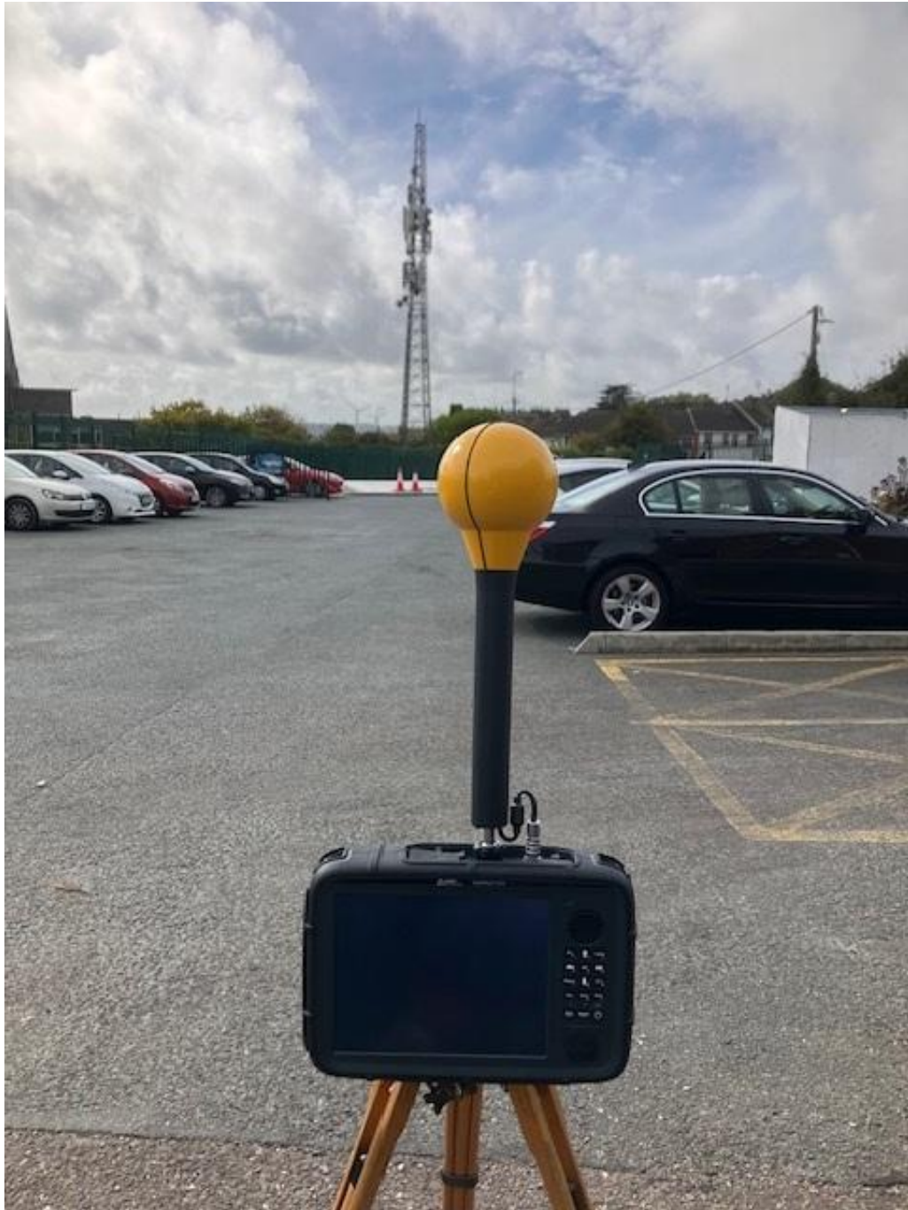
Photo 2. Frequency selective measurement location looking towards antennas
