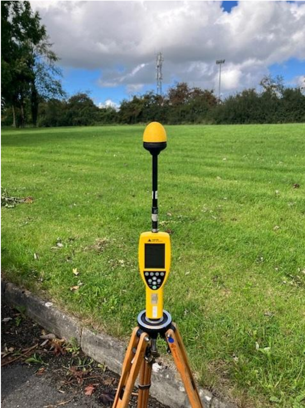
Photo 1. Broadband Measurement location looking towards antennas
