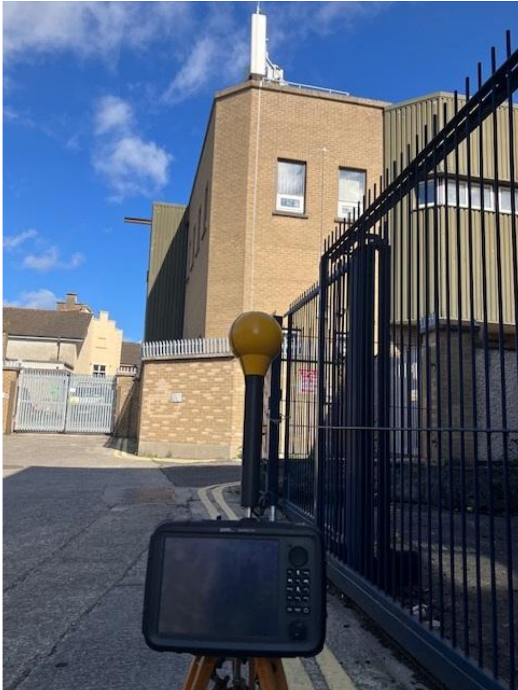
Photo 2. Frequency selective measurement location looking towards antennas
