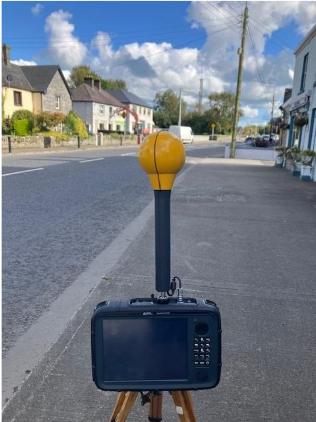
Photo 2. Frequency selective measurement location looking towards antennas
