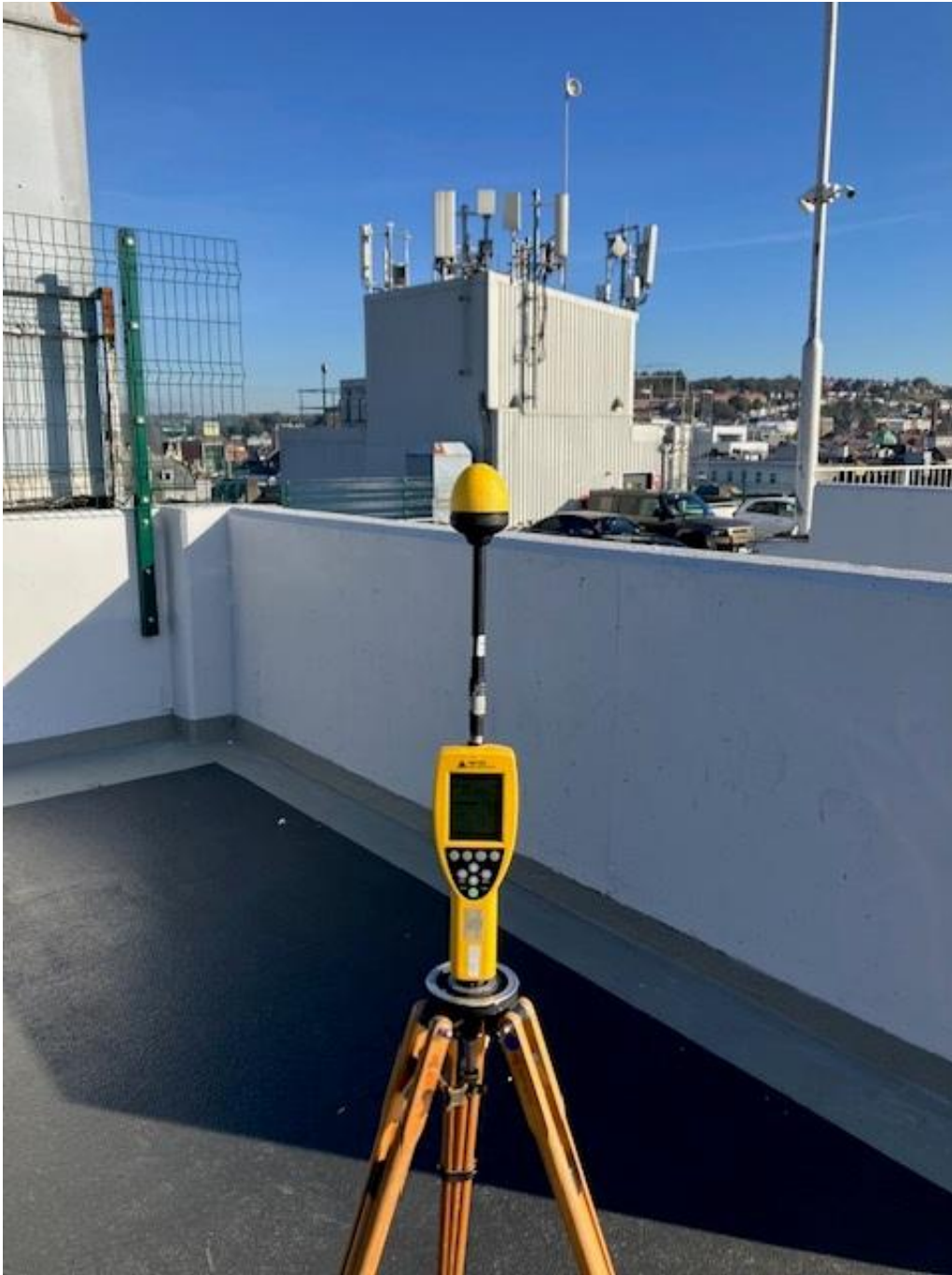
Photo 1. Broadband Measurement location looking towards antennas
