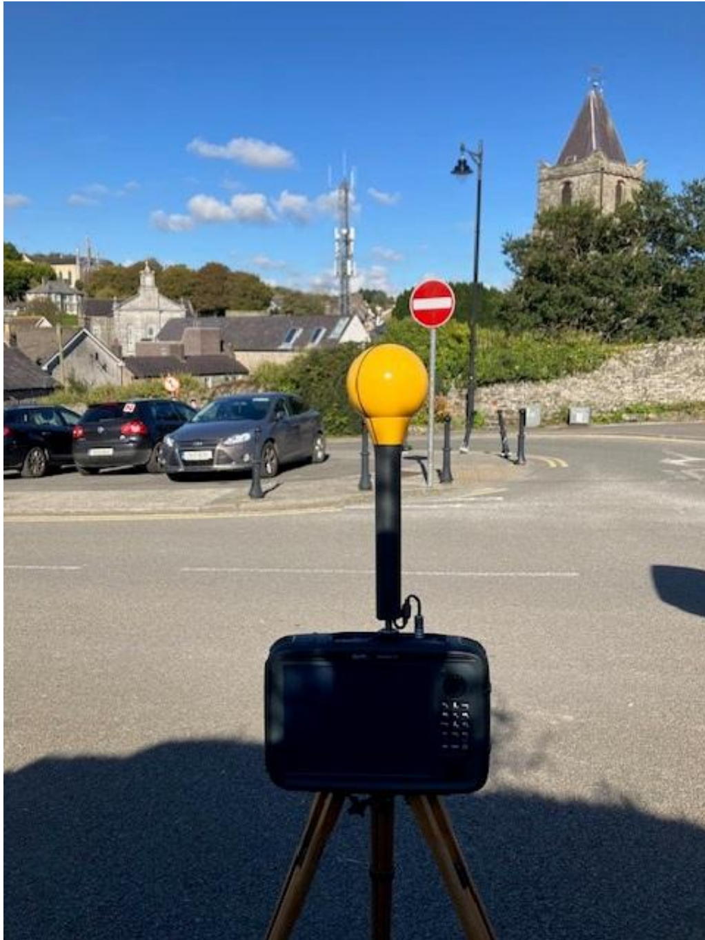
Photo 2. Frequency selective measurement location looking towards antennas
