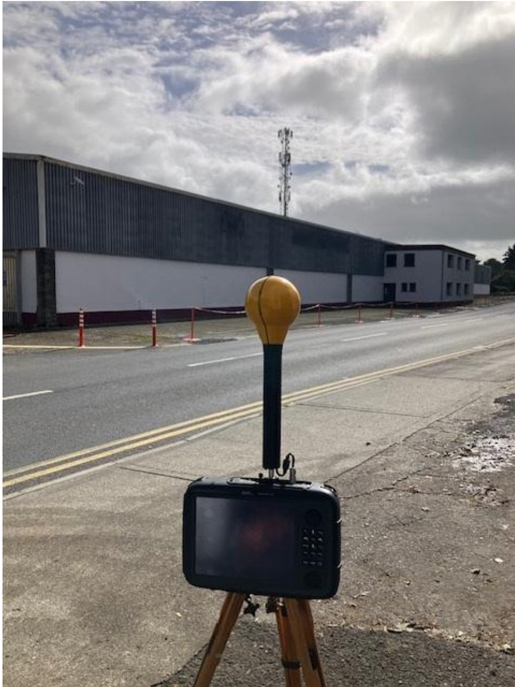
Photo 2. Frequency selective measurement location looking towards antennas
