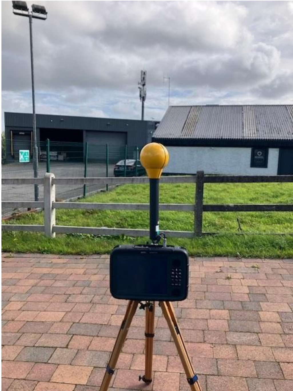
Photo 2. Frequency selective measurement location looking towards antennas
