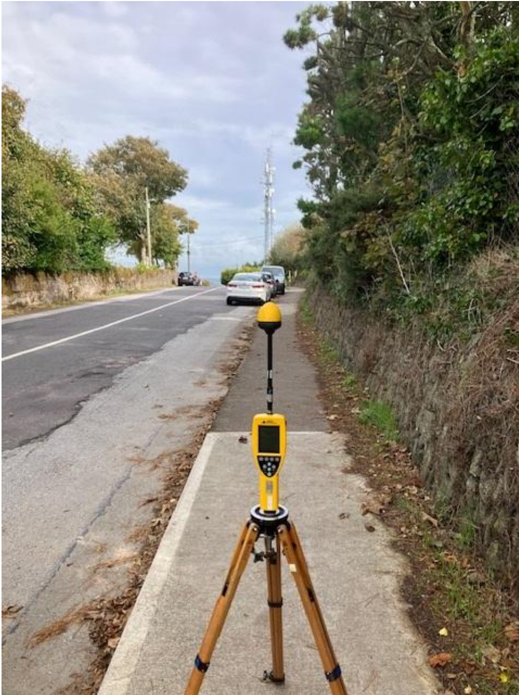
Photo 1. Broadband Measurement location looking towards antennas
