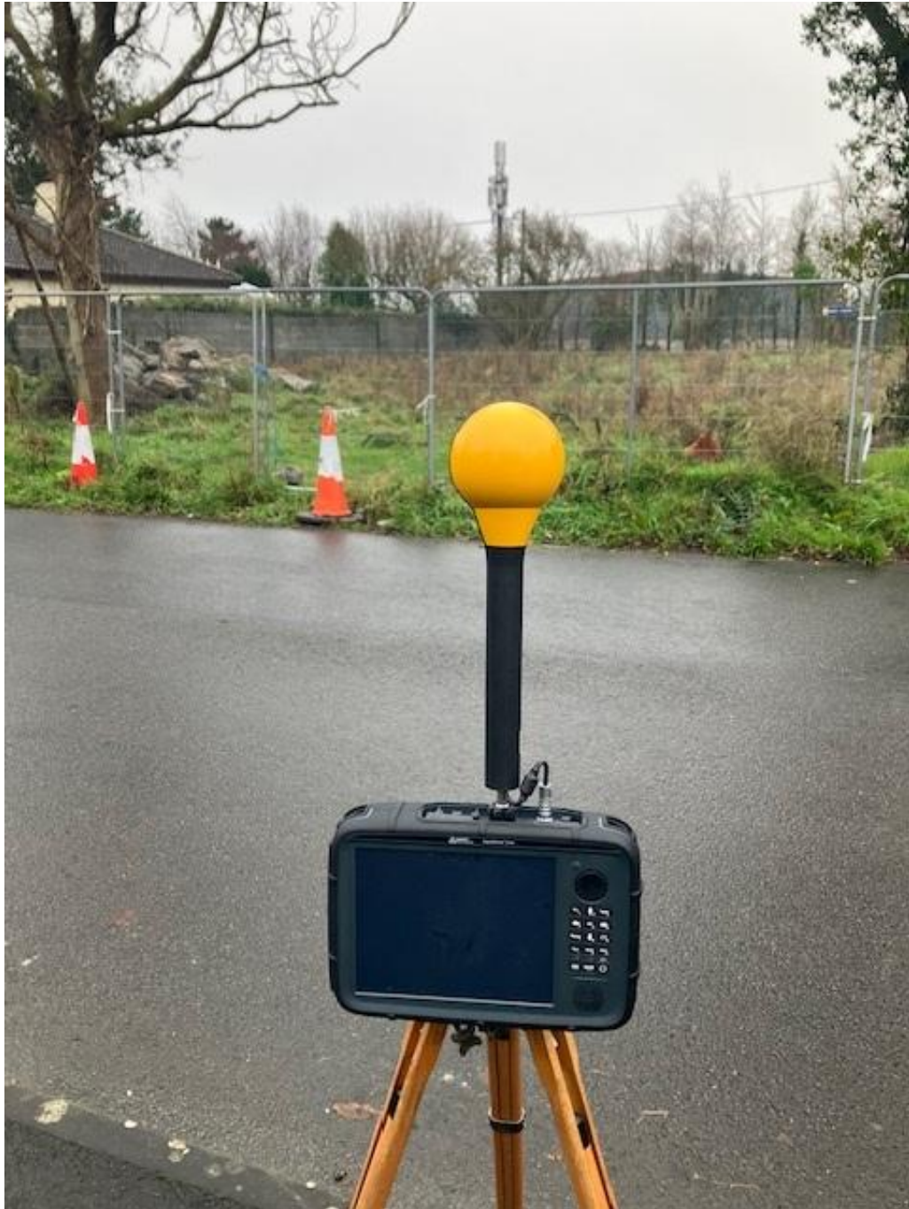
Photo 2. Frequency selective measurement location looking towards antennas
